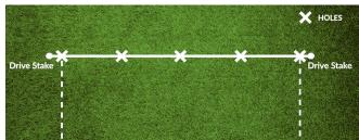
To ensure the posts are in a straight line, begin by setting your drive stakes past the furthest ends of your fence line and stretch the string between them. Determine the location of your first post and mark out each of the holes. Depending on your style of fence, the most common distances between posts are either 6' or 8'. Mark on the ground where each post will be placed.
